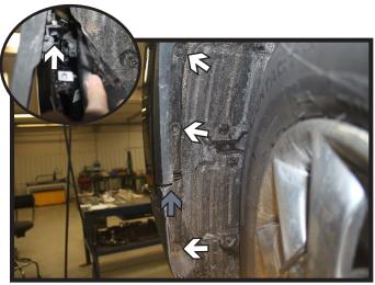
3. Using a 8MM socket, remove the three (3) screws from the edge of the wheel well. Using a 7MM socket, remove the one (1) screw at the fascia/trim joint (gray). Using a 10MM socket, remove the screw behind the trim (inset). Do this on both sides of the vehicle.
