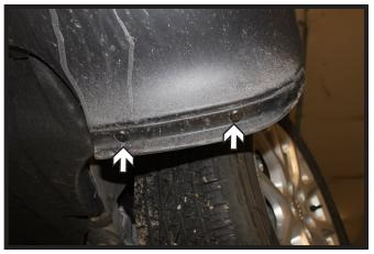
14. Using a 1/4" drill bit, ream out the existing rivet holes. Install the new plastic rivets into the underside of the fascia, where the factory rivets were removed.
