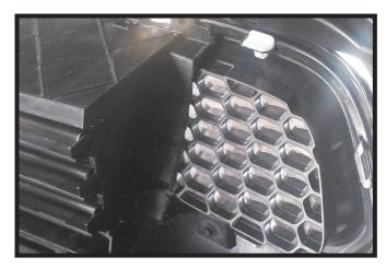
12. **Shutter Models:** The plastic surrounding the outer grille areas must be trimmed to expose the grill behind. Follow the protrusion straight down leaving the areas next to the screws intact. Do this on both sides of the fascia.
