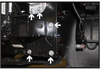
6. Using a 15MM socket, remove the three (3) bolts from the frame extension and two (2) bolts from the bottom side of the bumper (white). Using a 10MM socket, remove the nut from the fascia extension (gray). Do this on both sides of the vehicle. The extensions will not be reinstalled.
