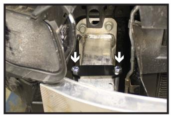
8. Install the support plate and bolts on top of the bumper thru the baseplate. Start the nuts onto the bolts. Fully tighten the frame and bumper bolts in the previous step then the bumper support bolts. Do this on both sides of the vehicle.
