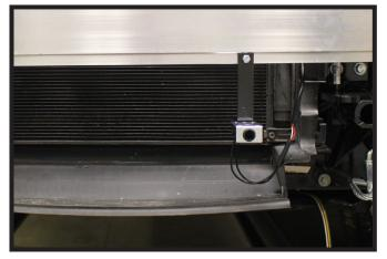
10. **Optional:** If installing a breakaway, drill a 1/4" hole thru the bumper lip in the desired location of the breakaway. Attach the bracket to the bumper with the 1/4" x 2" bolt and 1/4" lock nut. Attach the breakaway to the bracket with a 1/4"-20 x 3/4" bolt and 1/4" lock nut.
