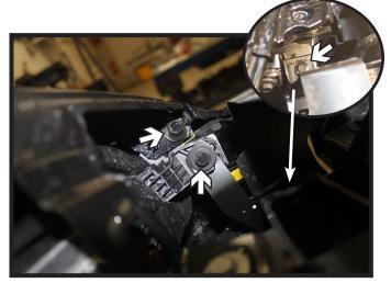
2. Using a 10MM socket, remove the three (3) screws from the backside of the fascia next to the fender. There are two (2) in the corner and one (1) directly below the bracket (inset). Do this on both sides of the vehicle.
