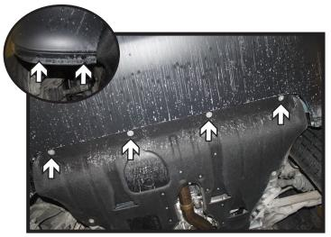
4. Remove the four (4) rivets from the underside corners of the fascia (inset). There are two (2) on each side. Using a 10MM socket, remove the four (4) screws from the middle portion of the fascia.
